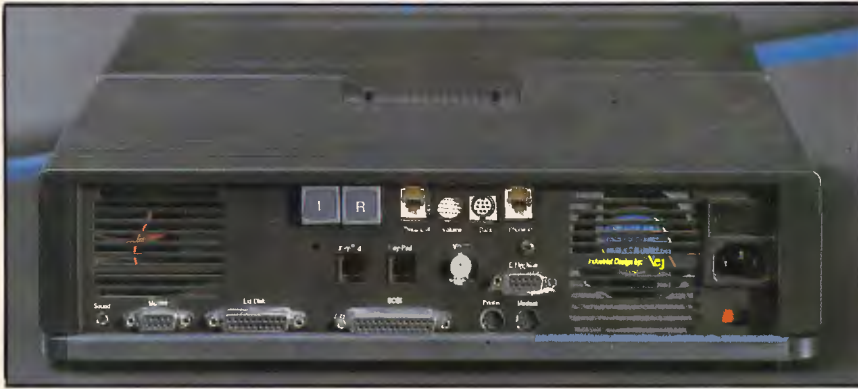
The rear of the Dynamac has been utilised to the limit. Most ports have been inherited from the Mac Plus, with additional slots for an internal modem and networking facilities
