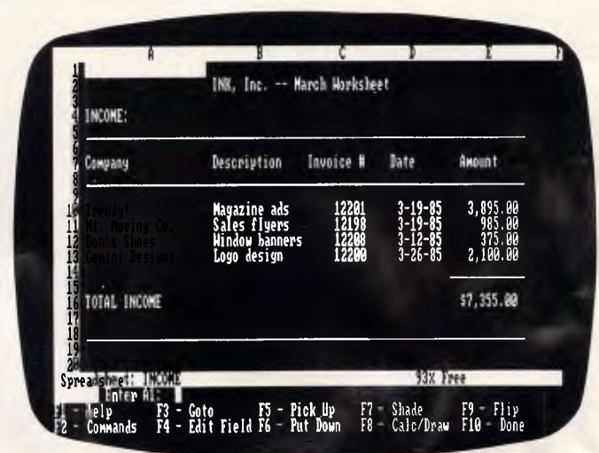
If memory permits, Ability will handle a spreadsheet of 9999 rows by 702 columns. Sideways printing is built in. Functions and formulas can be included in word-processing documents
