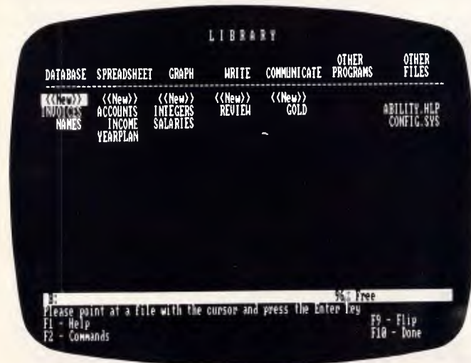
Creating a new file or using an existing one is simply a matter of selecting an option from the library screen. The column heading tells Ability which application program you want to load
