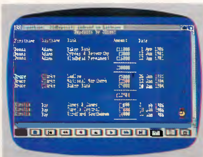
The result of applying a query on an example file — a table summary showing numeric fields
