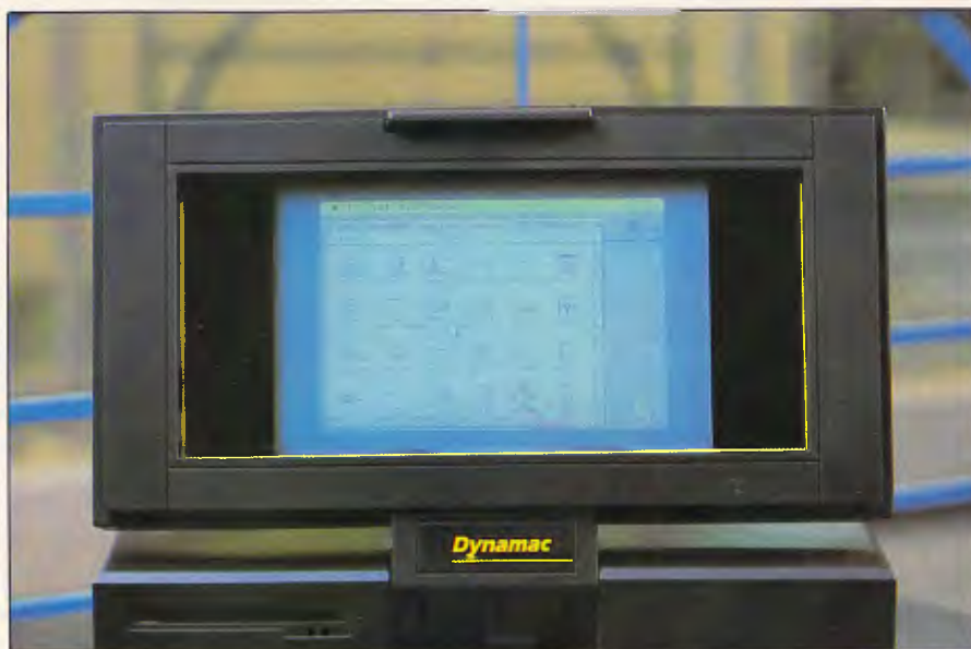
At 640×400 pixels, the Dynamac's power-hungry electroluminescent screen is 46 per cent bigger than the standard Macintosh unit
